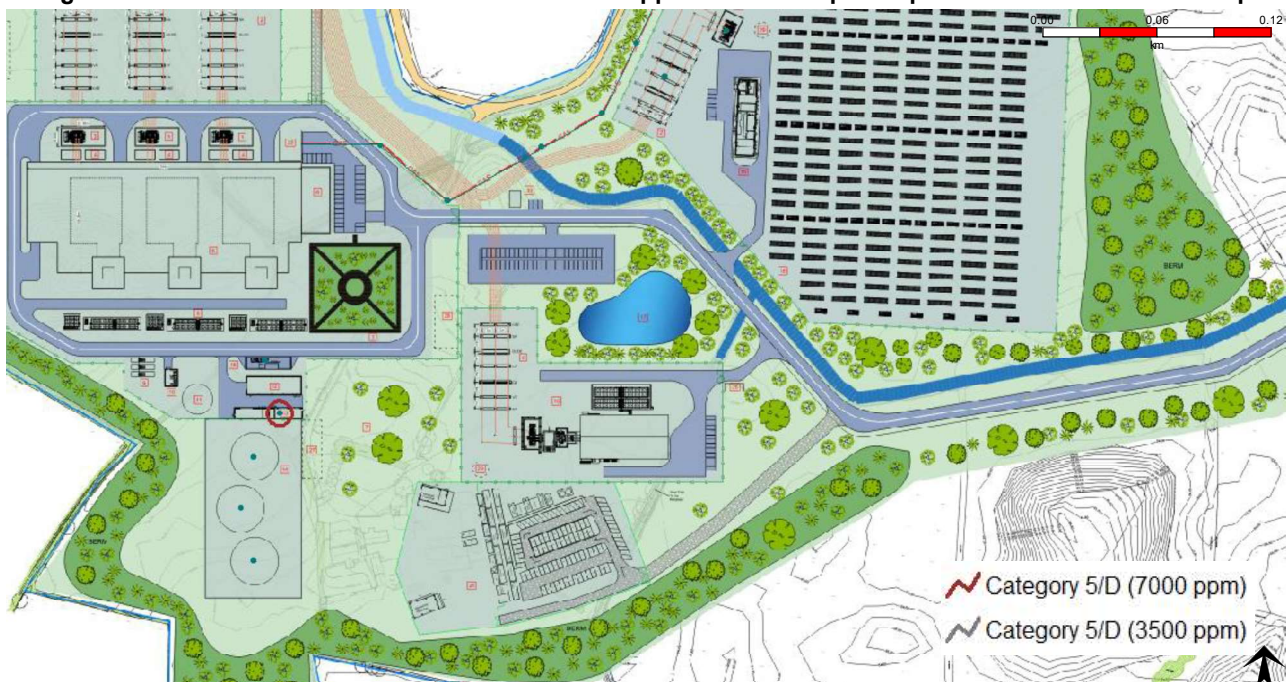
Figure 5-13: Flash Fire at 5/D for both 2500 and 5000 ppm for catastrophic rupture of Diesel Transfer Pump
