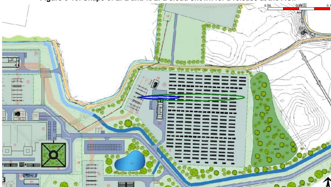
Figure 5-15: Shape of LFL and 1/2 LFL cloud shown for a release at the AGI.
